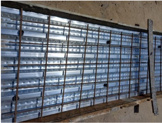
Figure 7 Specimen before pouring concrete
