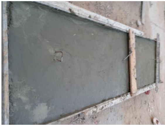
Figure 8 Specimen after pouring concrete
