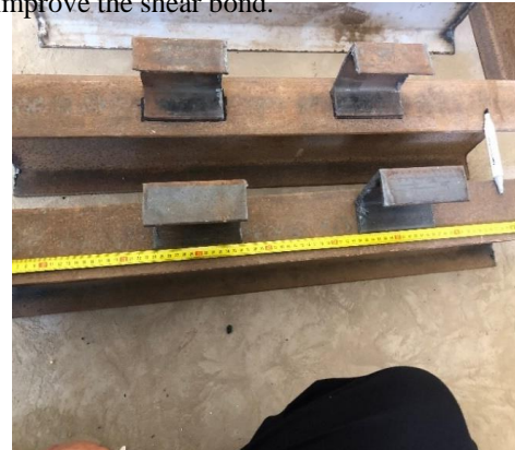
Figure 2 Arrangement of shear connectors
